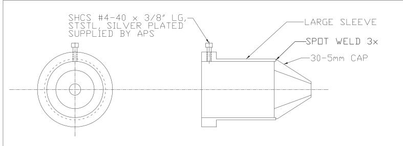
THIS COMPONENT IS PART OF AN ASSEMBLY INTENDED FOR ULTRA HIGH VACUUM (UHV) SERVICE. THE USE OF SILICONE, SULPHUR, PHOSPHORUS OR HALOGEN BASED CUTTING FLUIDS AND ABRASIVES IS PROHIBITED. USE TRIMSOL OR APPROVED EQUIVALENT LUBRICANT.
